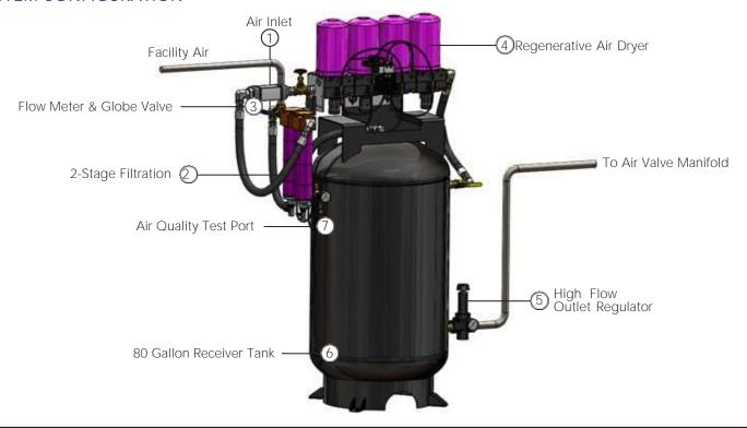
Pretreated air enters the regenerative dryer where dew points and relative humidity are lowered down to -40°F and .01% RH. Tsunami technology features self-regenerating towers to eliminate the need for manually change desiccant. This level of air quality prevents the chance of moisture creation during the supercooling process.
