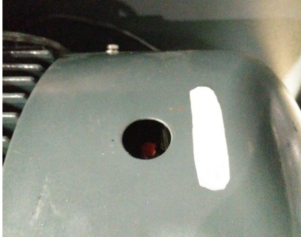
Fig. 37: Example: motor bearing grease port
