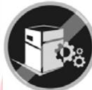
Danger hazard; It's absolutely forbidden to operate the machine when the parts (under pressure or electric panels) are not in place or have been tampered with and changed.
