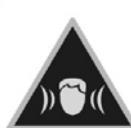
Danger hazard: Machine level noise could be higher than 85 dBA. It is mandatory to install the machine in dedicated area where people are not normally present. The installer and/or the user is responsible for correct installation of the dryer, in order to prevent noise propagation to the near work environment. The installer and/or the user is also responsible for the safety signs affixing into installation site.
