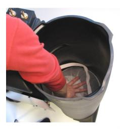
Push the element down untill all the trapped air has escaped out of the carbon element.
