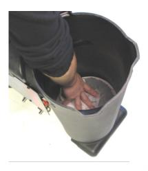
(Push the element down untill all the trapped air has escaped out of the element).
