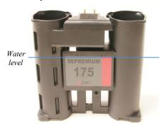
Tip: spraying water over the black element in tower 2 before filling the housing 5 prevents carbon dust from spreading.
