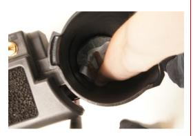
(Push the element down untill all the trapped air has escaped out of the element).
