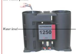
Tip: spraying water over the black element in tower 2 before filling the housing prevents carbon dust from spreading.
