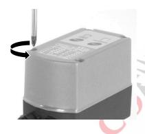
2. Place the 4 batteries and close the housing by replacing the 4 housing screws.
