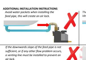
The feed pipe must be horizontal or ideally at a downwards slope (>1°).
