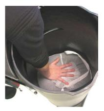
Push the elements down until all the trapped air has escaped out of the carbon elements.
