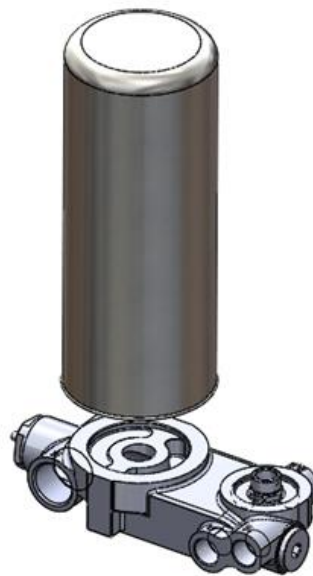
Figure 22 Separator Element Replacement
