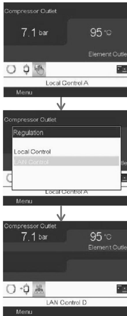
Flowchart how to integrate the compressors into the LAN
