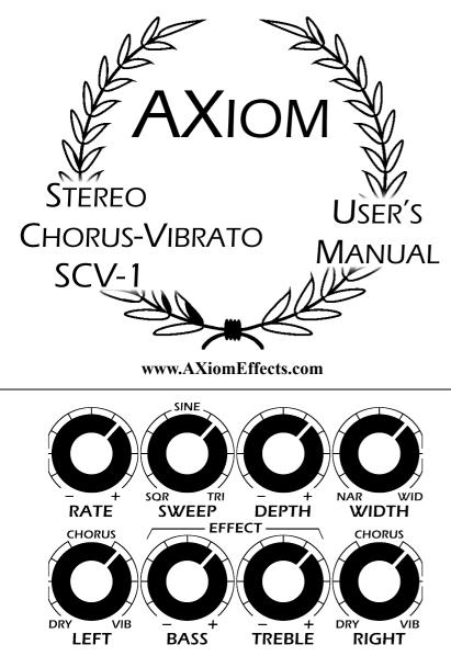
**RATE:** Increases the sweep rate of the modulation as the knob is turned clockwise.
