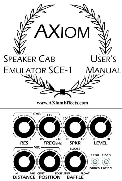
**RES:** Increases cabinet resonance as the knob is turned clockwise. **FREQ(Hz):** Adjusts the resonance frequency from 85 Hz to 210 Hz as the knob is turned clockwise. In general, larger cabs have lower resonant frequencies, 4x12 cabs resonate around 120 Hz, and smaller cabs resonate at higher frequencies - though this is influenced by speaker type and cab design. **SPKR:** Adjusts the speaker size from 8" to 15" as the knob is turned clockwise. Larger speakers exhibit stronger resonance.
