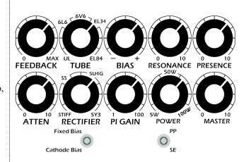
**FEEDBACK:** Increases the internal negative feedback level as the knob is turned clockwise (CW). This increases clean headroom and reduces distortion and compression.
