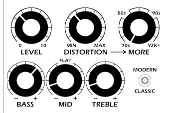
**LEVEL:** Increases the output volume level as the knob is turned clockwise.
