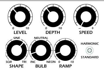
**LEVEL:** Increases the output volume level as the knob is turned clockwise. **DEPTH:** Increases the intensity of the tremolo effect as the knob is turned clockwise. In the fully counter-clockwise position there will be no effect at all, allowing the CT-1 to be used as a completely transparent clean boost.
