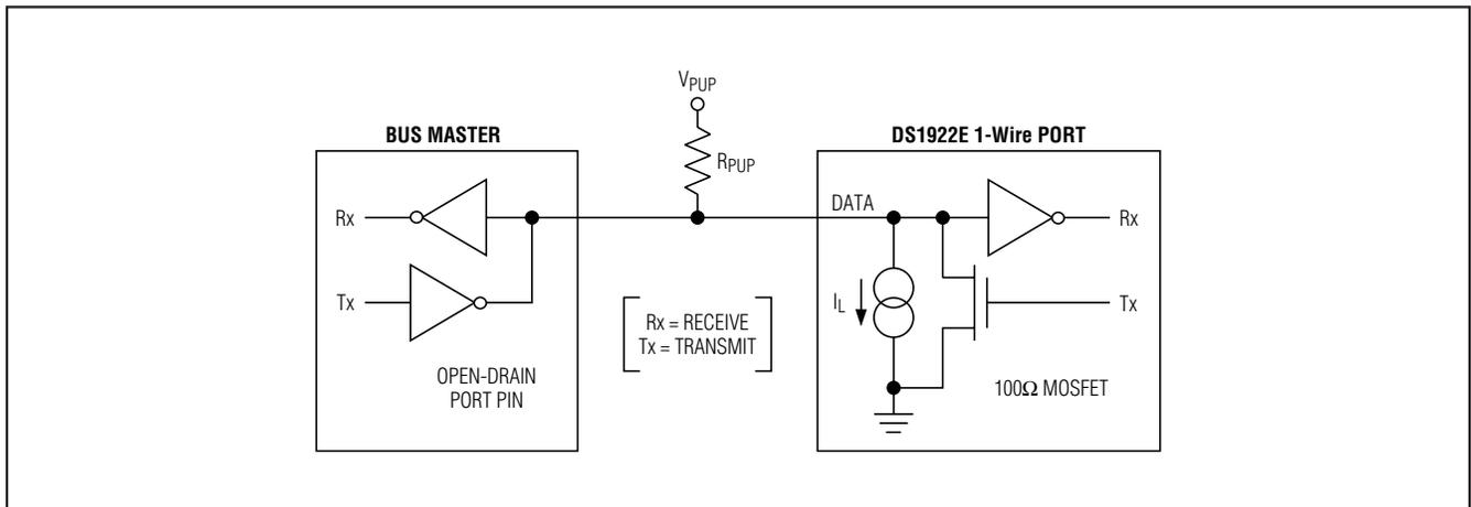
Figure 10. Hardware Configuration
