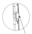
The outstanding point of the rear flying plate indicates the current angle.
