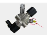
**2)** Using backup wrench on body nut to install defuel hose. *Torque to 30 inch pounds.*
