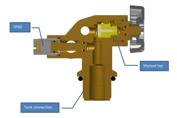
The Pressure-Relief-Device, thermally activated, is based on a fusible plug made from an eutectic alloy (Indium-Bismuth alloy, lead-free).
