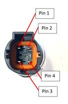
Pin 1 and 4 are for the mid pressure point (250psi). Contacts will close when the pressure is reached. Used for triggering the fan relay.
