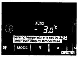
In this case, depress HOT switch ( $\triangle$ ) or COLD switch in step 6. Each time the switch is depressed, displayed temperature will change by 0.5°C. In this way, sensed temperature can be varied in the range from +3.0 to -3.0°C. (Example)
