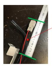
Install 2 pin Deutsch connector on lift pump wiring. Tail should be around 150mm long from the bolt to the end of the connector. Positive wire needs to go to position 1, and negative to position 2 (As per picture).
