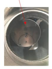
Step 4: Install lift pump. Place the bolt through the 6mm hole on the top of the surge tank tube, install washer and nut.
