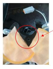
Step 7: Install the pump strainers supplied, install the retaining clips. When pumps are positioned correctly in the hanger, the hole in the center of the lower plate should be visible and clear of obstructions. The edges of the strainers will need to be folded slightly on the spring side.
