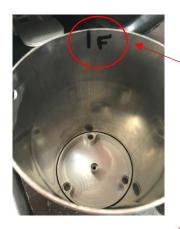
Step 3: Install surge tank tube into the fuel tank. The tube has an "F" with a line to show the front or forward position. Install the tube with the F towards the front of the car. Once the tube is inside the tank, move it to the right to create space for the lift pump.
