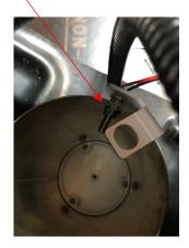
Step 5: Place the lift pump hose through the hole on the bracket so the hose points down into the tube. Retrieve the connector for the pump and for the fuel level sender. Position the tube so it is centered and in line with the access hole and the F is at the front.
