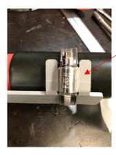
Position clamp as per the picture and slide pump into the holder.
