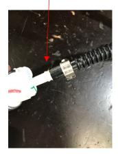
Install the pumps into the hanger, the hoses will be looped, and position the pumps between the two plates. Once everything is in its spot, install the feet and tighten them with your fingers. The pump inlets should be positioned as per the picture.
