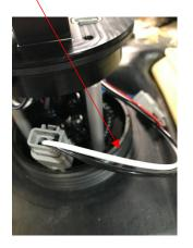
Step 10: Lower the assembly into position (some slight rotation to the left and right may be necessary), until the feet and the springs engage into their pockets in the base of the tube. Do not use force, they should find their way. The assembly should sit up 4-8mm and the springs should be felt when pushing down on the hat. When those conditions are met, push down on the hat, and install the locking ring. You will notice that the hanger comes with a special seal.
