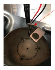
Temporarily install the lift pump assembly onto the surge tank tube (bolt on bracket goes into the 6mm hole on the tube). Rotate the pump and set the height so the pump sits 0.5mm-1mm off the bench. This is important. Tighten the clamp holding the pump.
