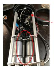
Step 6: Install the pumps into the hanger. You cannot install a pump directly below the return port, as it will not fit into the tube.
