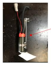
Step 1: Assemble lift pump as per the picture. (If your brackets look different, scroll down to Step 1A)
