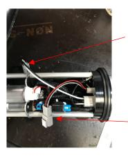
Step 8: Ensure the fuel sender wiring and the lift pump wiring are out of the way and not tangled.
