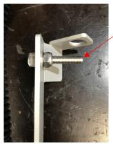
Install bolt, washer, and locknut.
