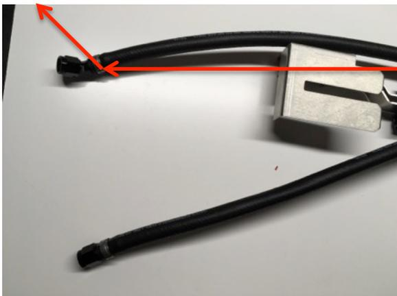
Left pump hose should have the 45 degree fitting in line with the pump and facing up
