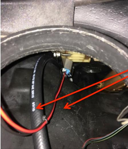
Hose needs to be on the left hand side of the arm, and the wiring can come straight up.
