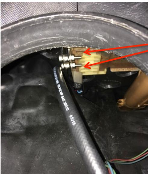
Washer, nut and washer installed on both bolts.
