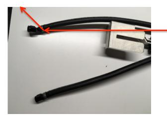
Left pump hose should have the 45 degree fitting in line with the pump and facing up
