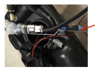
Connect the wring to the left pump now or it will be difficult to do in the tank. Step 5: Insert the left arm and pump assembly inside the tank and slide the arm onto the bolts on the holding bracket.
