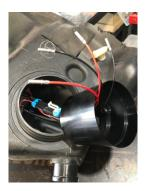
Step 3: Install the middle section of the surge tank, ensure the wires and the hoses are placed through the centre, then connect the middle section to the lower section. Some rotating and wiggling may be required as they can be a tight fit.
