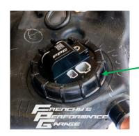
Step 13: Install hat into position and tighten lock ring.
