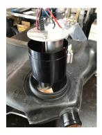
Step 1: Slide lower section (the unit with the lift pump on it) into the fuel tank, rotate the assembly to allow it to find its way in. This method is for the Walbro 255 and 460/525 pumps. \*\*For the longer BKS1000 pump, read additional step below\*\*.
