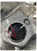
Step 7: Install the last section of the surge tank, feed the wires through the smallest hole (you need to feed them one at a time), the hose through the 21mm hole, and lower the last section into the tank.
