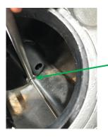
Step 10: Wind threaded rod out by hand, all the way until it touches the tank wall and as tight as you can with your fingers. Wiggle the surge tank and check rod tension. This will ensure that there is minimal movement inside the tank. Tighten the nut with a 10mm spanner to secure the rod in place.
