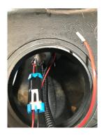
Step 2: Engage the foot of the surge tank into the factory plastic holder. Do not push it all the way at this stage.
