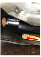
Step 5: Push the assembly all the way into the factory plastic holder. Make sure it goes in straight, it's can be a tight fit.
