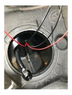
Step 8: Engage the last section onto the middle section, some rotating and wiggling may be required. Make sure nothing gets caught. The threaded rod should be placed towards the tank floor and the wires at the top as pictured.
