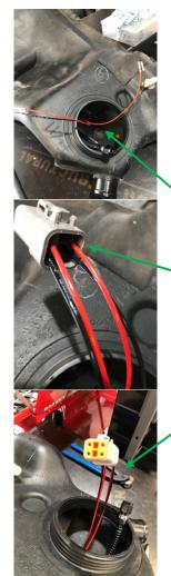
Step 9: Install the wires into the 4 pin Deutsch plug supplied. The seal has been removed on purpose as it does not handle fuel.
