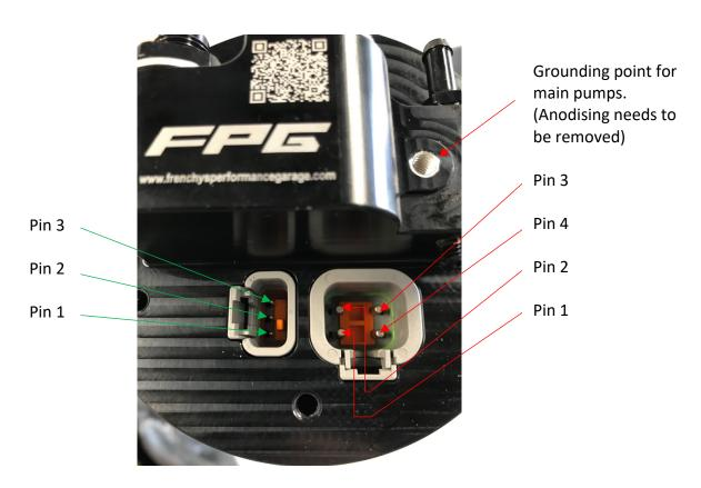
4 Pin Large Deutsch Connector (DTP4): Used to power pumps
