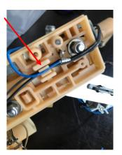
Install and slide the FPG sender into position, and fit the small cable tie supplied behind. This will stop the sender from accidently popping out.
