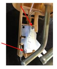
Install washers and locknuts supplied, tighten them evenly until the plate is mounted flat and straight. Do not overtighten.
