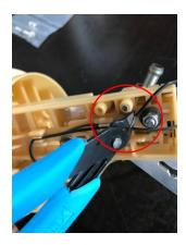
Cut the factory sender wire on both sides of the solder joint. Strip the ends (5-6mm)
