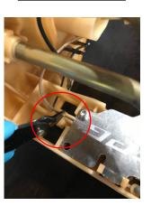
Strip the end of the factory wiring (5-6mm), shorten one of the blue wires on the FPG sender and strip the end (5-6mm) work out the length carefully. Crimp the factory and the blue wire together with the crimp supplied. Clip the wiring back into the holding fingers.
