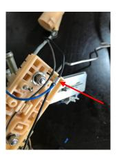
Shorten and strip the end of the remaining FPG sender blue wire. Crimp the 2 factory wires and the blue wire together using the crimp supplied. Clip the wires back into the factory spot.
