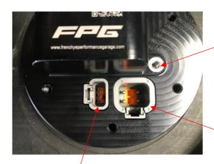
DTM3: Fuel level sender. Connect the 3 factory wires in the same order as the OEM connector. Pin 1 Green/Blue Pin 2 Red Pin 3 Black
