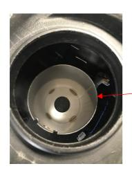
Step 3: Install the cylinder in the fuel tank. Make sure it is sitting on the base plate and clear of obstructions.
