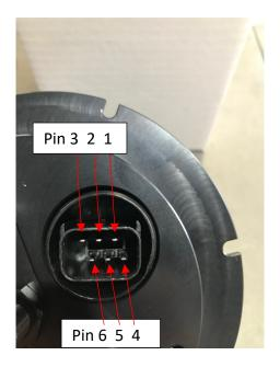
Note: The red secondary lock needs to be removed for the underside connector. We also recommend removing the seals inside the tank as they could react with certain fuel types and blends.
