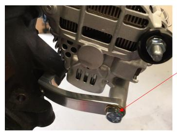
Tighten the bolt on the back brace to 30LbFt (40N.m). This ensures that the alternator is now square to the block.
