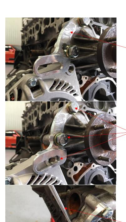
Install the adjuster bracket onto the water pump as per the picture. Leave the top bolt finger tight, and do not engage the bottom bolt into the slot as yet. Loosen the main pivot bolt so the alternator can move back and forth. This will allow you to install the belt onto the pulley and gives you maximum slack. Install the belt on.
