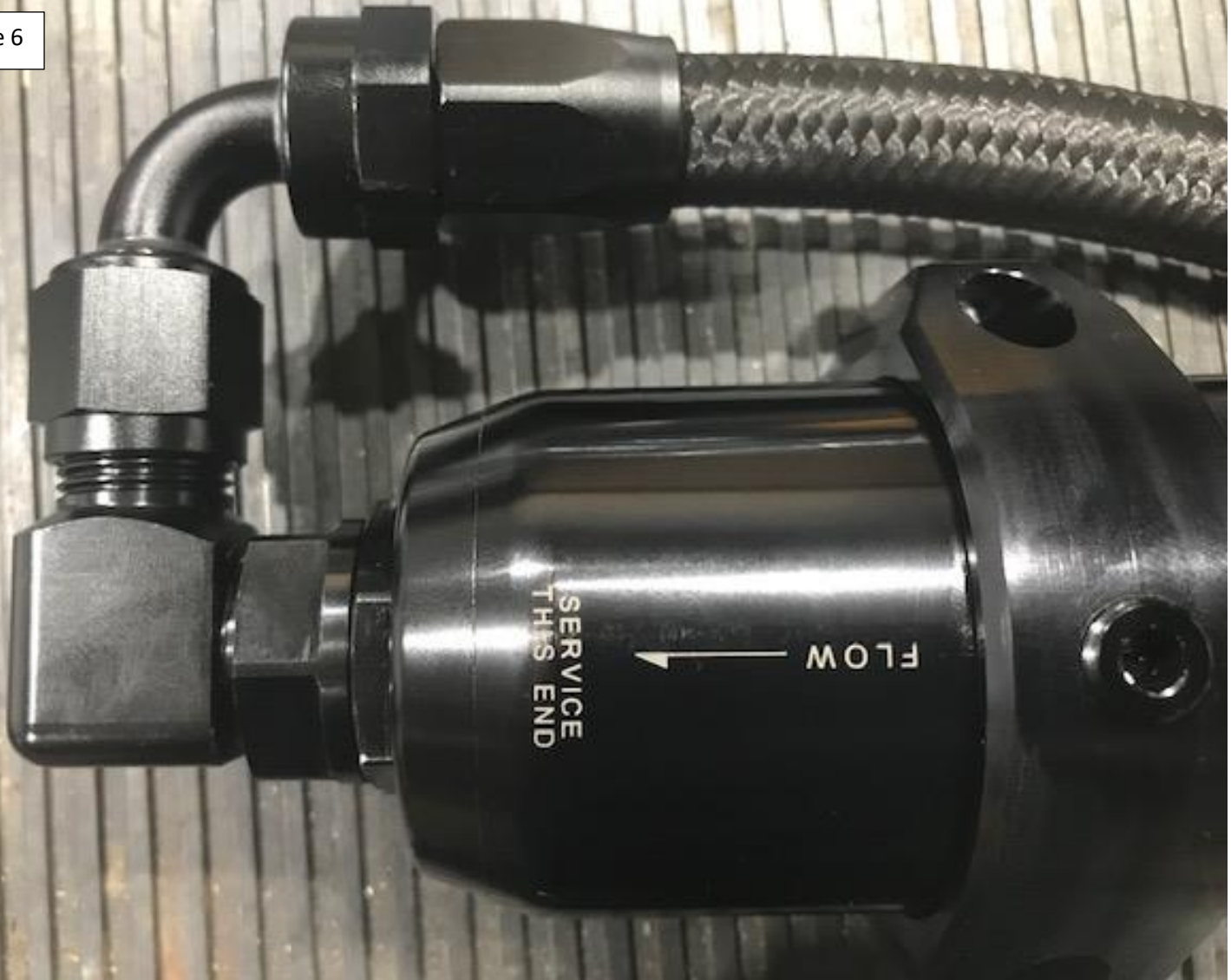
Figure 6 showing fitting and filter setup, note that the 1/8 NPT plug is used in the center of the billet bracket to keep filter from rotating, do not over tighten!
