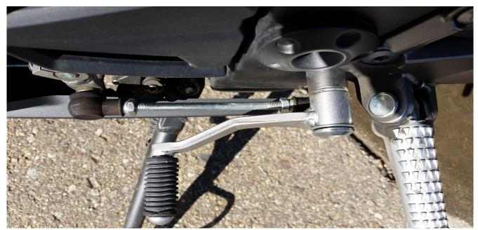
You can see that the shift rod screws directly into the rose joints. The likelihood of finding this style shift rod in the new length you will need is low. So each HM Quickshifter comes with a set of stub screws to use should you need to install a newer style shift rod like the one pictured in our first example above.
