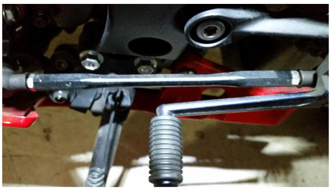
You can see the black rubber covers on each of the rose joints, the locking nuts, and the black shift rod between the two silver locking nuts.
