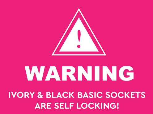
Do not assemble the sockets with the terminal inside before it is wired. The terminal will lock the socket permanently
