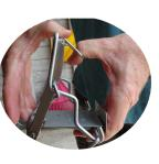
Pull both thumbs apart descending the top cross bar towards the safety and trigger catch, opening the jaws.
