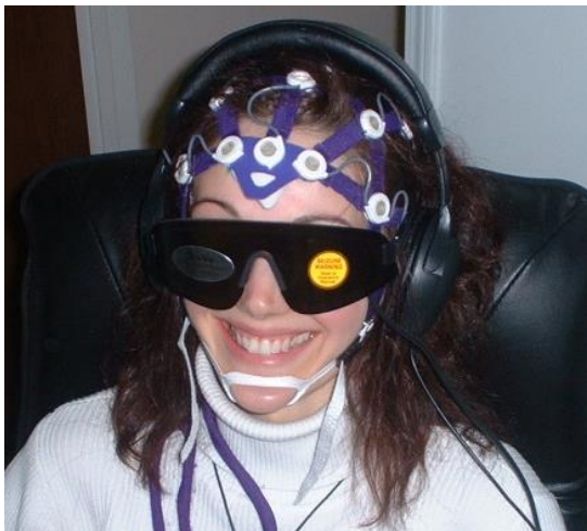
Figure 12. Person Wearing a 10-20 Electrode Cap While Using AVE.
