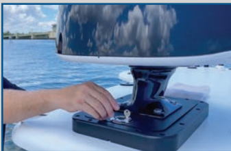
Step 1: Unlock latch to remove lid
