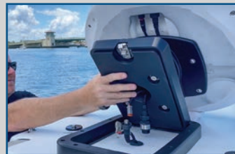
Step 3: Disconnect the cables
