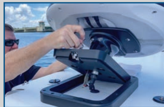
Step 2: Unlatch and fold the electronics AFT
