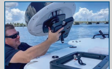
Step 4: Remove the mount/ electronics
