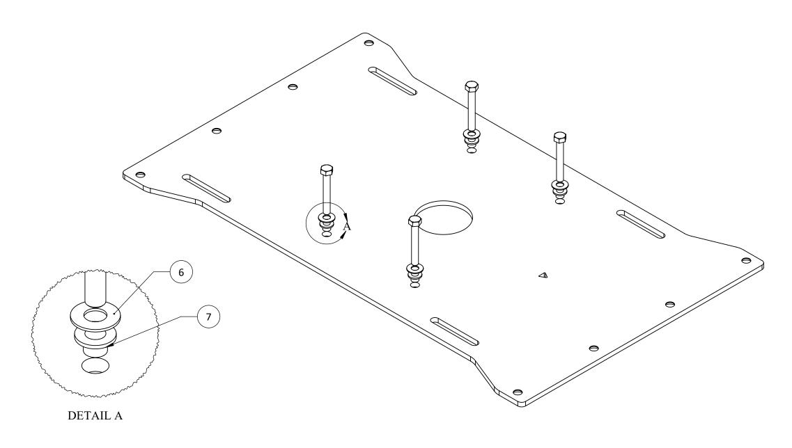
Bolt one end cap to the Aluminum plate using all of items (4) and (5
