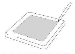
Remove the template and drill the hole(s) that will secure your electronic instrument.
