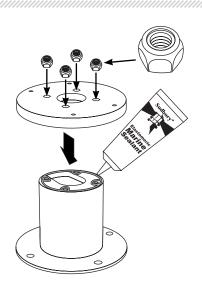
Secure the ADASL8 plate to the PM5FN8P using the four ¼-20x7/8" bolts.
