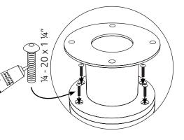
Apply marine adhesive sealant to the base of the mount.
