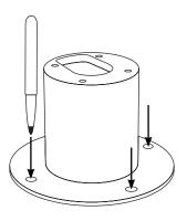
Use a drill bit to drill the four bolt holes.
