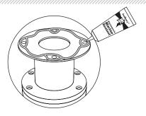
Route the cables through the cable hole on the surface and mount the assembly, be sure that all four mounting holes line up.
