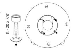
Apply marine adhesive sealant to the top of the ADASL8 plate.
