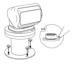
Use your own hardware to secure the mount to the surface. Be sure to apply marine adhesive sealant to the threads of the bolts.
