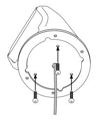
Apply marine adhesive sealant to the PM5FN8P as shown. Insert four 1420LNUT nuts into the ADASL8 plate. Note this may have already been done for you.
