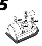
Drill pilot holes and secure the base. Apply marine sealant to the threads of the screws (optional).
