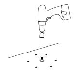
Bolt the camera to the Top Down Riser using the six bolts and washers.
