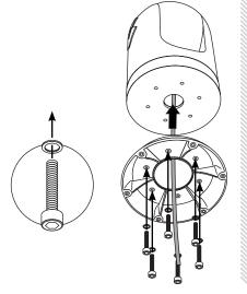
Note, when mounting the Sionyx Nightwave you will need to drill the cable hole in the FTDR3. You will also need to apply marine sealant in and around the slotted hole to keep water out.
