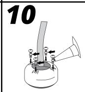
Apply marine sealant (optional) to the four allen head screws and tighten.
