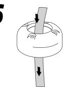
Slide the Cable Seal cover over the electronic cable.
