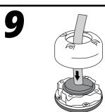
Slide the Cable Seal cover onto the plastic base making sure that all four bolt holes line up.
