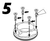
Drill pilot holes and secure the base. Apply marine sealant to the threads of the screws (optional).
