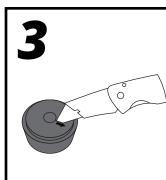
Using a sharp razor blade or knife, cut the tapered plug from the cable hole outward.
