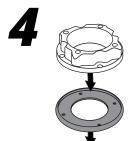
Place the plastic base onto the rubber base gasket. Be sure to line up the four screw holes.
