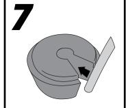
Wrap the tapered plug around the electronic cable.
