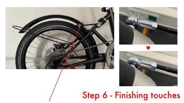
Make sure that the fasteners on the front end of the mudguard can move freely, i.e. the screws must not be locked with the nuts so tightly that the struts are clamped (which is also not necessary due to the self-locking nut). This is important so that the mudguard can move freely when folding the VELLO.
