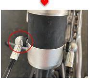
It is common for the mudguard to initially sit off-center. To fix this, vary the lengths of the struts by screwing the frame mounting ends in or out (maintain the minimum four turns!). You can also help a little manually (see <a href="here">here</a>).
