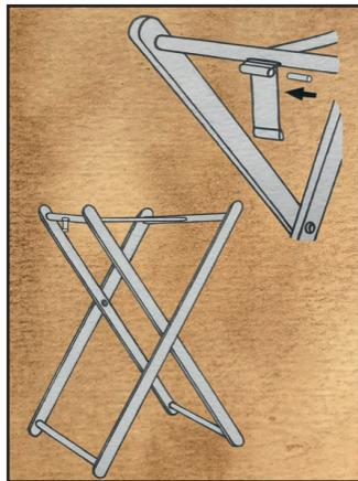
To raise the height insert the wooden cylinders inside the buttonholes showed in the picture above.
