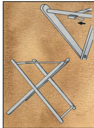
To lower the height, put the cylinders inside the buttonholes at both ends of the cotton band.
