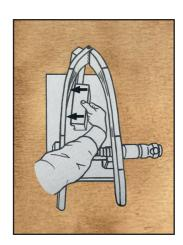
Put one or both the reductions on the inside side of ham holder. The two reductions adapt to the size of the product once sliced.
