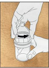
Unscrew the top glass dome in order to remove it.
