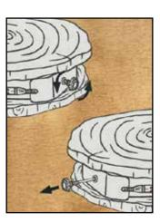
Remove the key turning counterclockwise.
