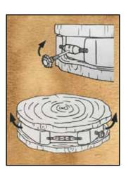
Insert the key in the hole of the mechanism and turn upwards to expand the iron band.
