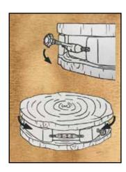
Turn downwards to tighten the iron band
