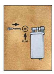
Drop the new flint down into the flint hole. Reinsert the spring into the hole and refasten the screw.
