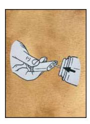
Reverse the lighter and refill using butane gas. Press the stem of the refill can directly onto the refill valve on the bottom of the lighter. Keep them in a straight position and press for about 5 seconds. М
